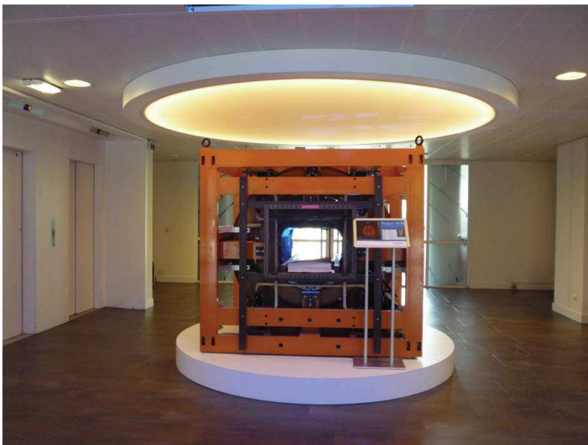
Figure 1.4 0.15 T resistive magnet used by Philips in the early development of MRI. Courtesy of Philips Healthcare.
